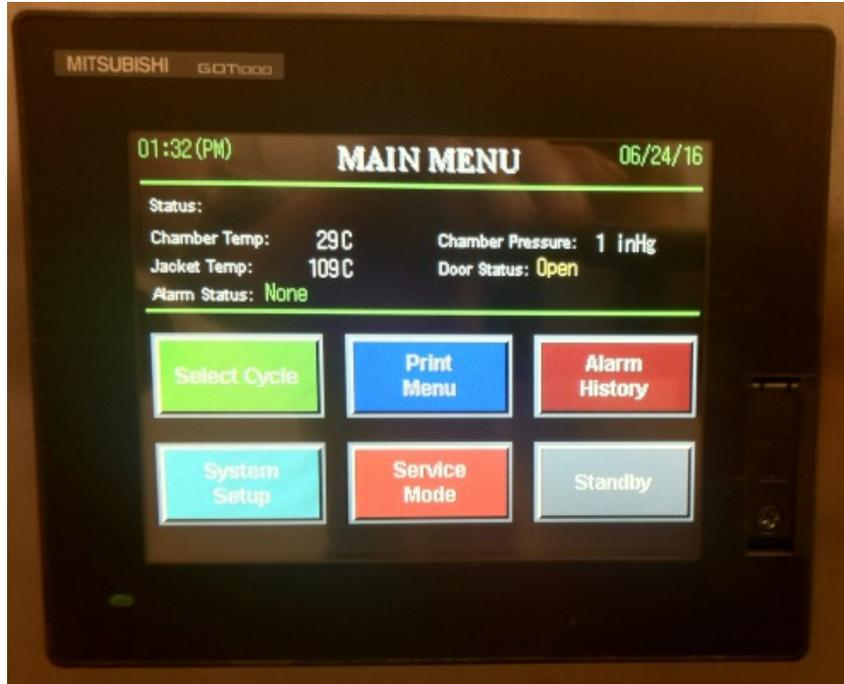
**Figure 2. Autoclave controller Main Menu screen**
